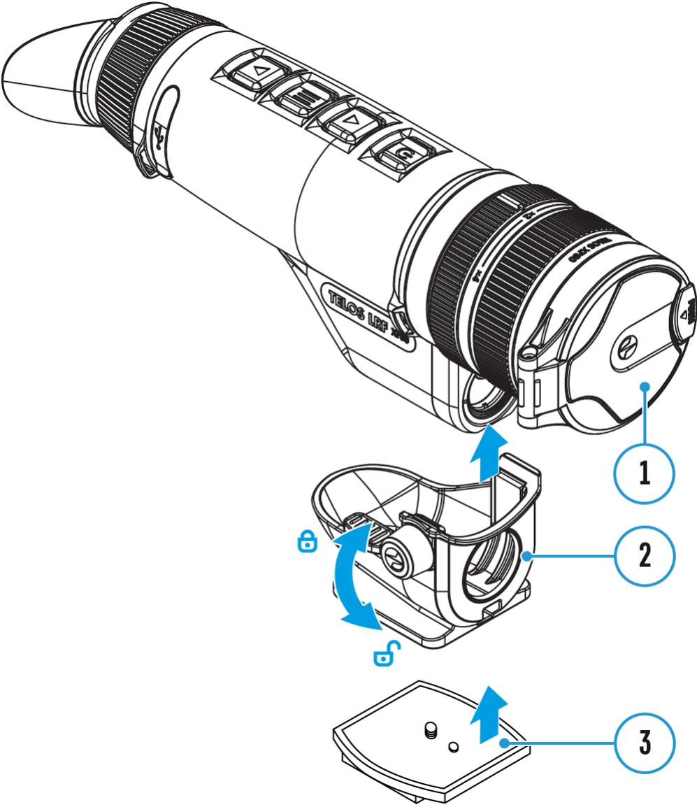
1. Screw the tripod adapter **(2)** onto the tripod mounting plate until it stops.
